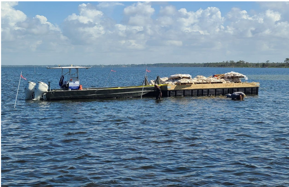
Figure 12. An aluminum barge was used to transport prepared sediment tubes to the restoration areas.
